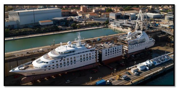
Caption: Windstar Cruises' Star Breeze is cut in two, with the new section inserted, at Fincantieri's Shipyard in Palermo.
